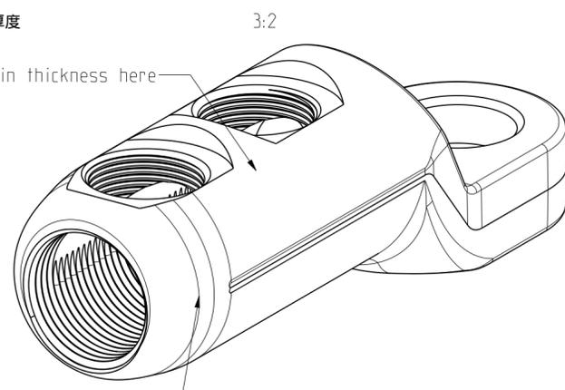
Smoothen forging burrs all around the part. Sharp edges are not allowed
